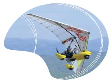
The double surface area pressurized to 40% of the iFun 16, associated with low twist and optimized profiles along the wingspan according to their respective angles of attack, allow it to display performance to rival many wings with an internal crossbeam! The sail also deserves its name D.S.E.T. (Double Surface External Transversal) rather than single surface, so much it differs from its class thanks to design and performance...
