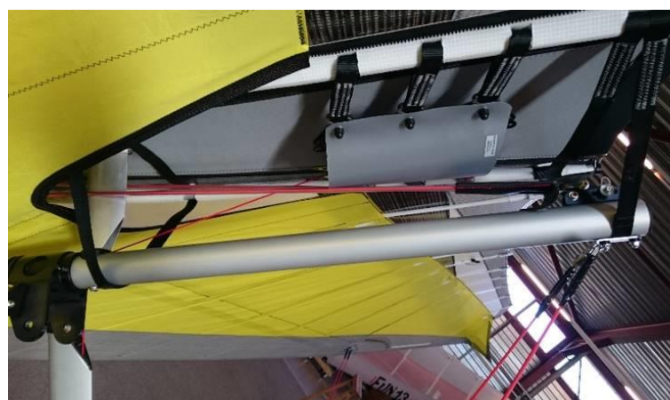
Figure 5-2 : Path of Tensioning Cables
