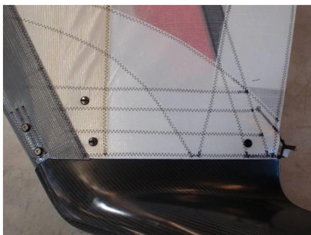
Figure 5-3 : Wing Tip Fin Fasteners
