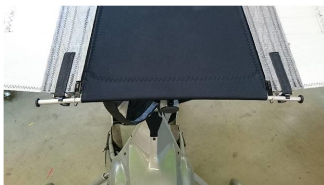
Figure 5-5 : Trailing edge tensioning batten
