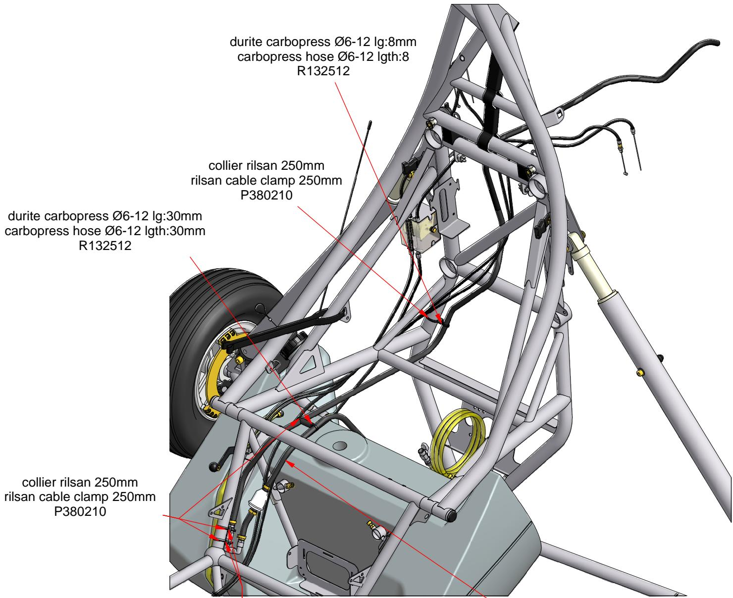
durite carbopress Ø6-12 lg:8mm
